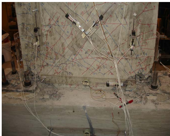
a) Specimen S8 at 2.1% drift
