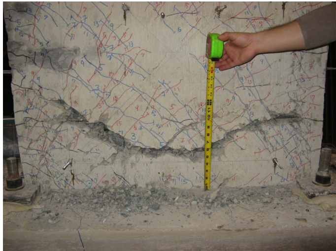
a) Specimen S9 at 2.1% drift
