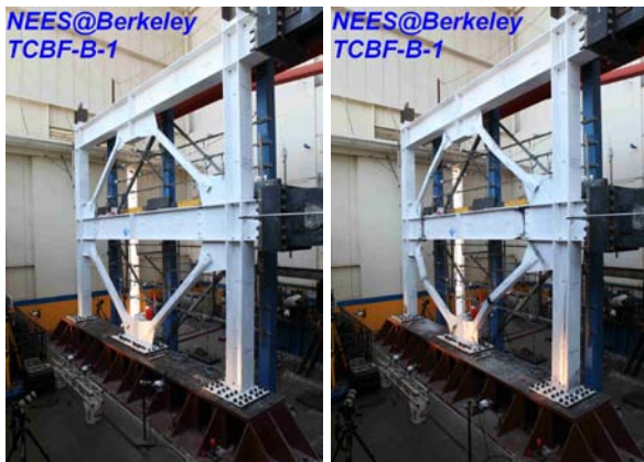
Figure 3. Specimen TCBF-B-1, before test (left), after test (right)
