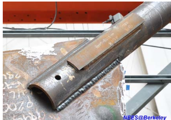
Figure 6. Detail view of reinforcing plate
