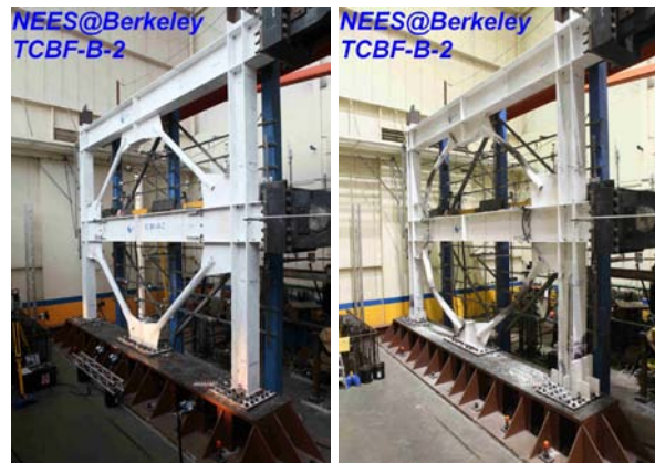
Figure 4. Specimen TCBF-B-2, before test (left), after test (right)
