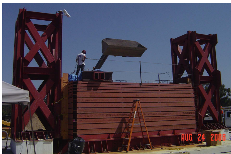
Figure 1. Soil container and restraining towers on shake table during backfilling.
