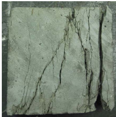
Figure 2. Typical failure surface of uniaxial compression plate specimen (a), and NM6 uniaxial compressive behavior (b).
