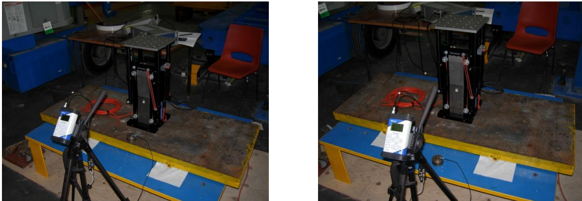
Figure 2. Set up showing the table, the surcharge and the shaker.
