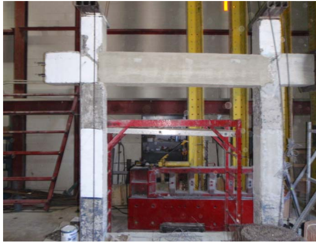
Figure 3. Repaired specimen BR-3R.
