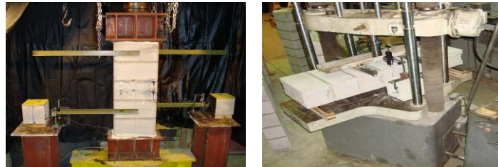
Figure 1. Tests for evaluating (left) compressive and (right) tensile strength of masonry assemblage
