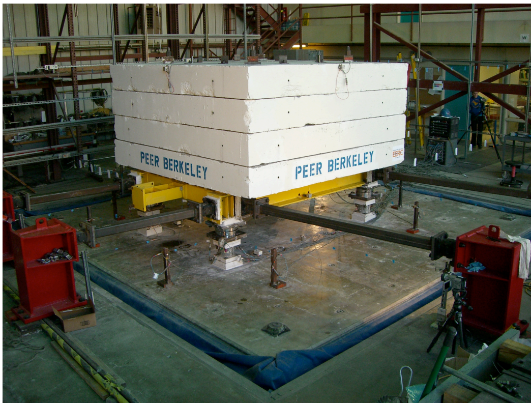
Figure 4. Rigid block experimental set-up at the UC Berkeley PEER Earthquake Simulator Laboratory.
