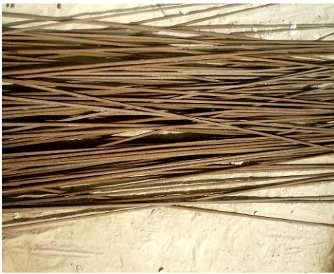
Figure 6. Improper maintenance of material (bars)
