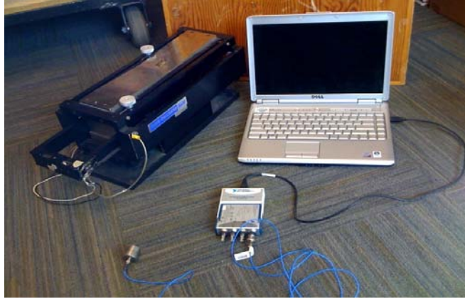
Figure 2: Test equipment (shaker, accelerometer, DAQ, computer).
