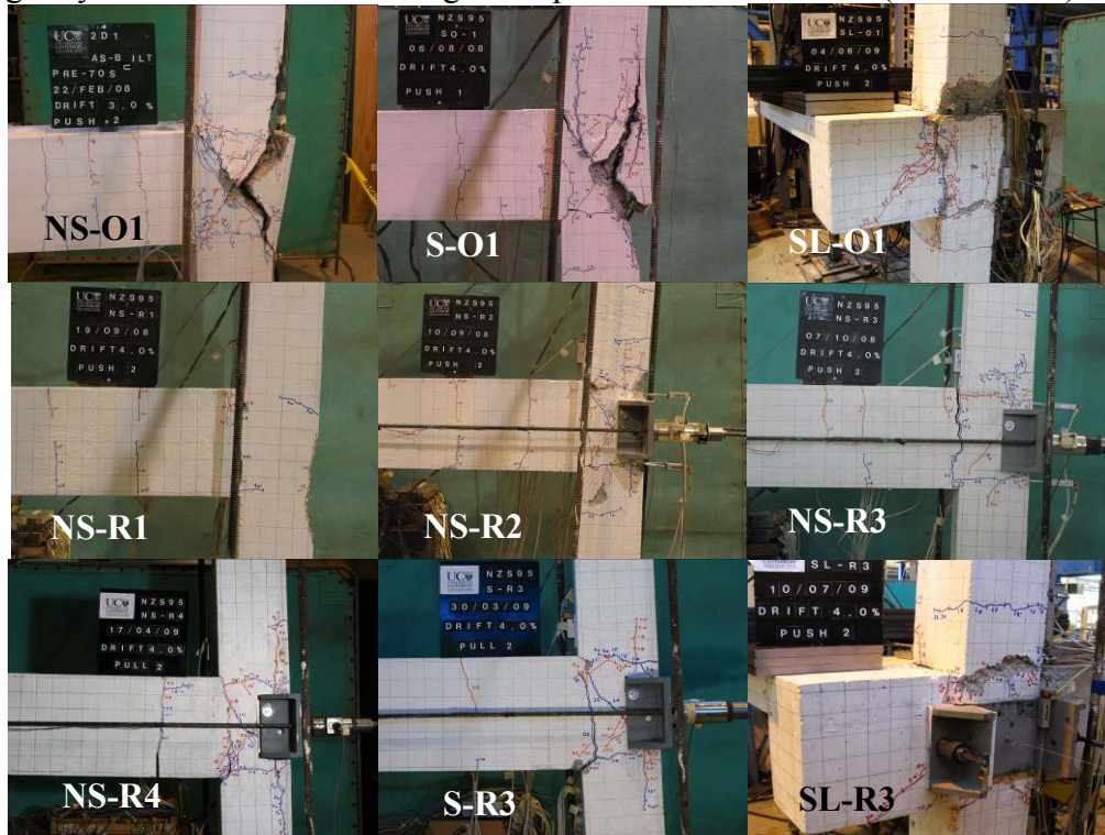
Figure 6. Failure and damage patterns at the end of the tests.
