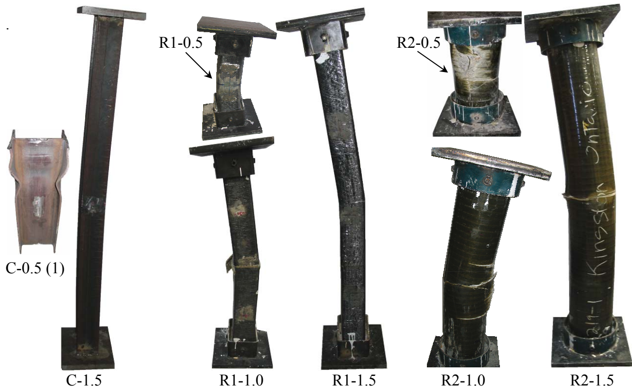
Figure 8. Failure modes of the tested columns
