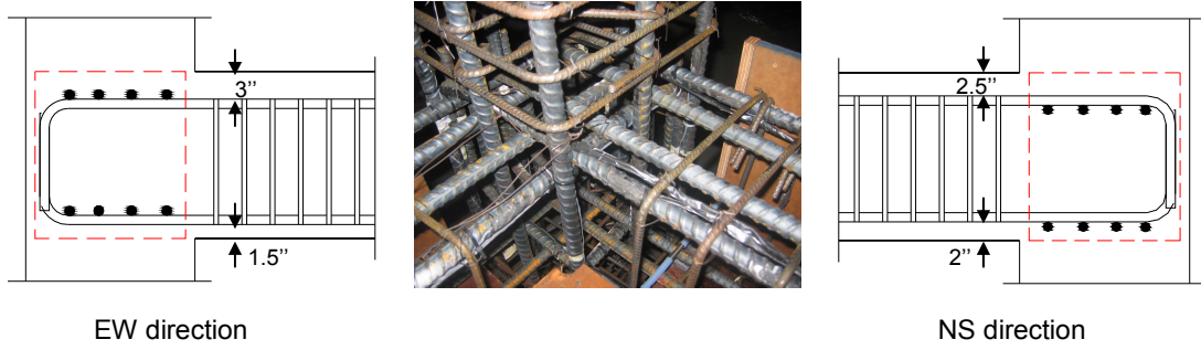
Figure 2. Placement of beam reinforcements in specimen SP1.
