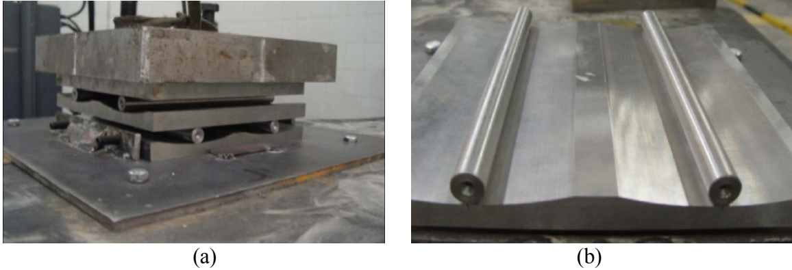
Figure 2. The proposed isolation system: (a) A set of the prototype sample under test, and (b) One pair of rolling rods on their concave beds
