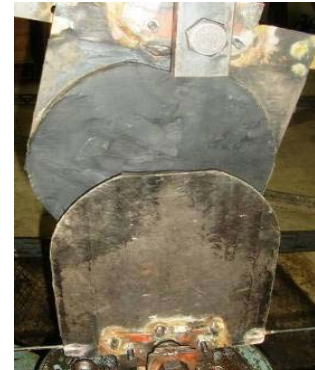
Figure 6. Comparison of the cyclic response for applied level of shear strain equal to 160% with equivalent test under monotonic loading for the cylindrical specimen of 250mm diameter (left). Failure of the 250mm cylindrical specimen (right).
