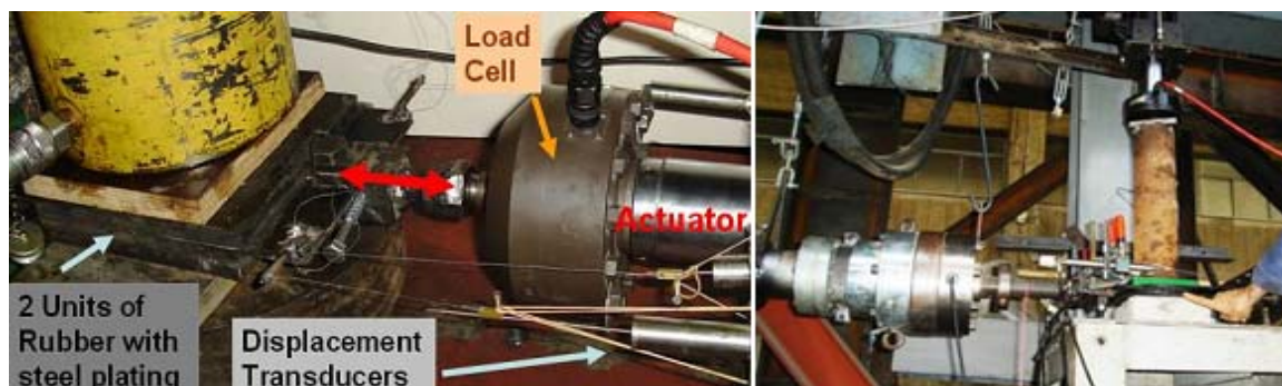
Figure 3. Loading arrangement of a unit slice (left) and cyclic shear strain imposed simultaneously with the application of the desired constant compressive force perpendicular to the bearing layers (right).
