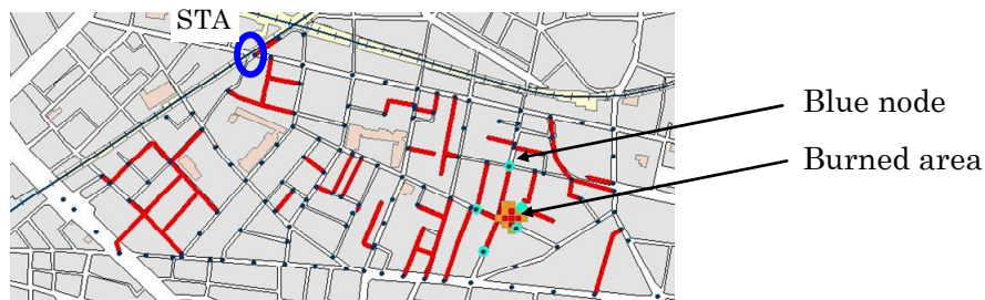
Figure 13 Possible points (green nodes) near the fire disaster area that a fire engine can reach.
