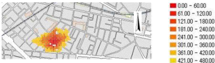
Figure 5 Simulated result of fire spreading from an ignited point.
