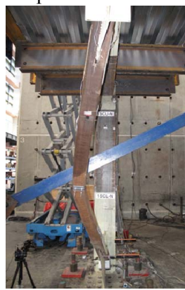
First Story Brace -1.39%
