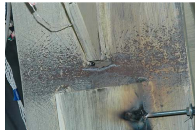
Tears in Mid-Span Knife Plate (+1.74%)
